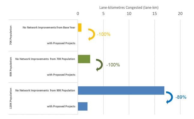
**Figure 4-31** is an indexed chart showing the relative growth in population, network lane-km and then the percentage of the network that is congested with and without the suggested network improvements over the assumed growth horizon. It is clear that without any improvements, the growth in congestion is significant, and that the suggested improvements provide a substantial reduction in levels of congestion across the network.
