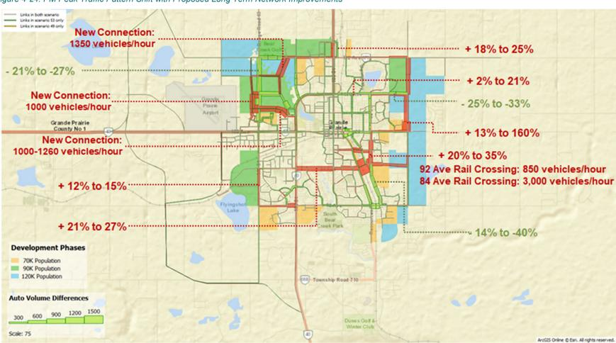
Figure 4-24: PM Peak Traffic Pattern Shift with Proposed Long Term Network Improvements
