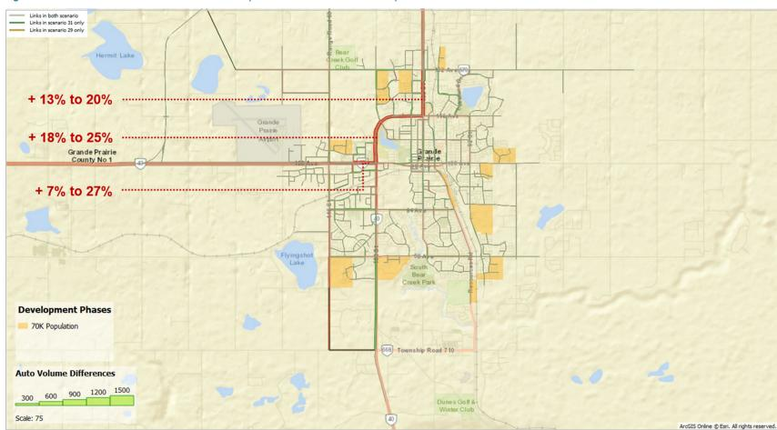
Figure 4-14: PM Peak Traffic Pattern Shift with Proposed Short Term Network Improvements
