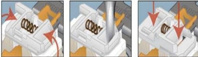
Shutters restrict access in closed position
